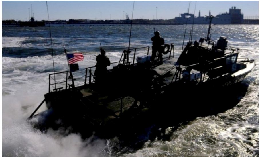
Figure 1: On 22 October 2010, the Navy conducted a full power demonstration of this alternative fuel-powered RCB-X running on a blend of 50 percent algae-based and 50 percent petroleum-based fuel, achieving a speed topping 44 knots ( about 52 miles per hour ).
